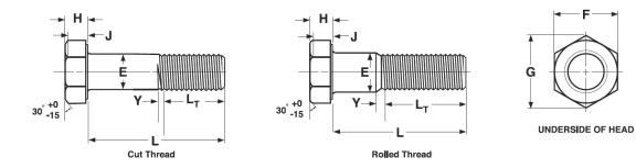
$\pm$ Length of a cap screw is measured from the underhead bearing surface to the extreme end of the screw.
