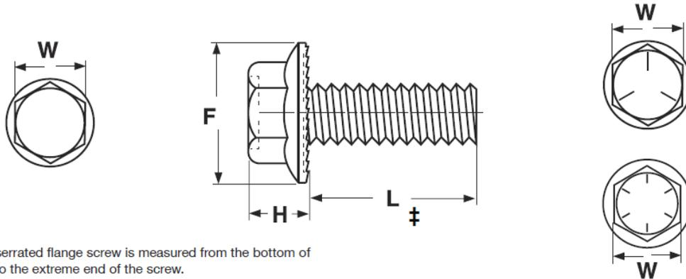
‡Length of a serrated flange screw is measured from the bottom of the serration to the extreme end of the screw.
